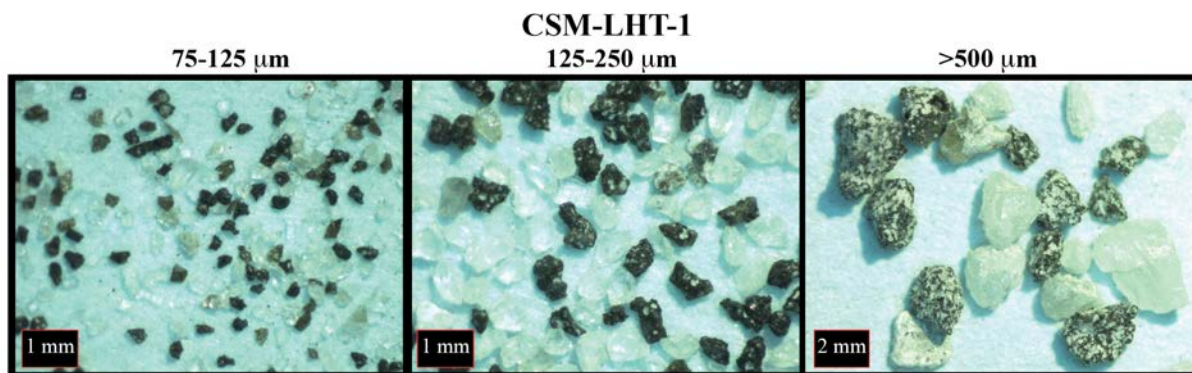
Figure 13: CSM Lunar Highland Simulant (CSM-LHT-1), shown at three different size fractions. The light particles are largely anorthosite and the dark particles are mainly basaltic glass.
